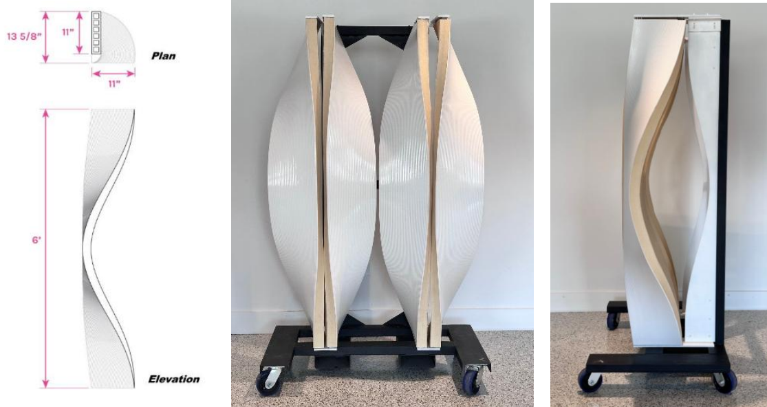
Figure 3. (Full-scale terracotta prototype in elevation and side view exhibiting the twisting geometry and minimal attachments)
